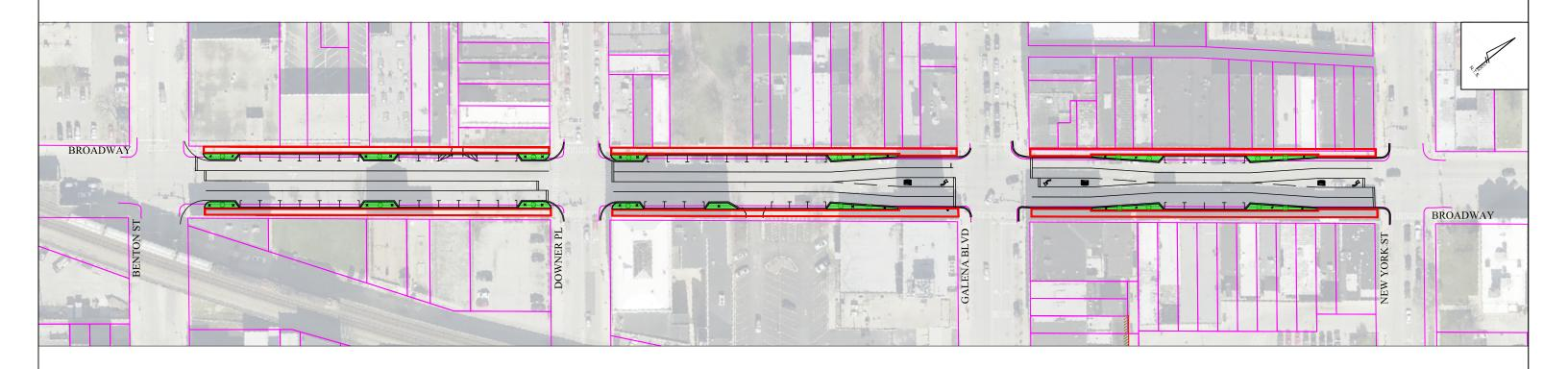
NOTE: ALL THROUGH LANES HAVE WIDTH OF 11' (9' EXISTING WIDTH) LEFT TURN BAYS HAVE WIDTH OF 10.5' (9' EXISTING WIDTH) ON STREET PARKING WIDTH OF 8' (8' EXISTING WIDTH)
