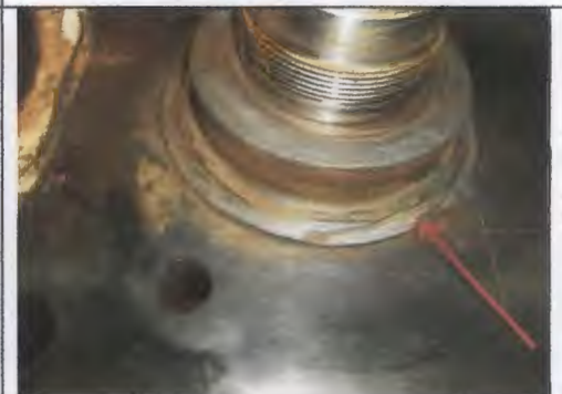
Erosion on top centering bracket.
