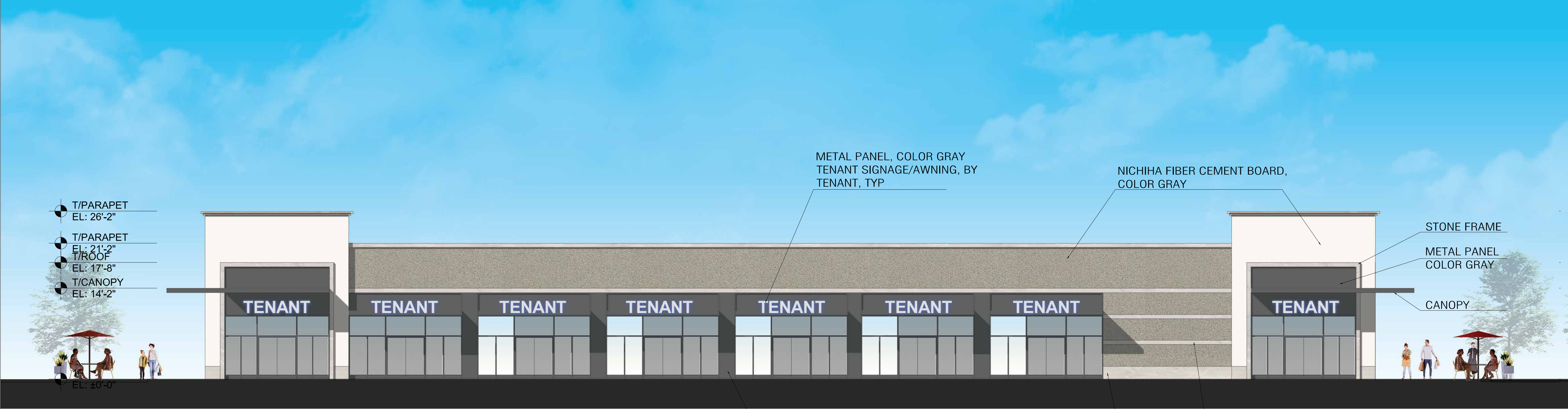
② BLDG 3 NORTH ELEVATION 1/8"=1'-0"
