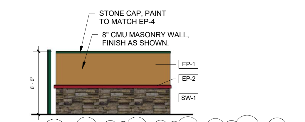
7 DUMPSTER ENCLOSURE - ELEVATION EAST A-2 3/16" = 1'-0"
