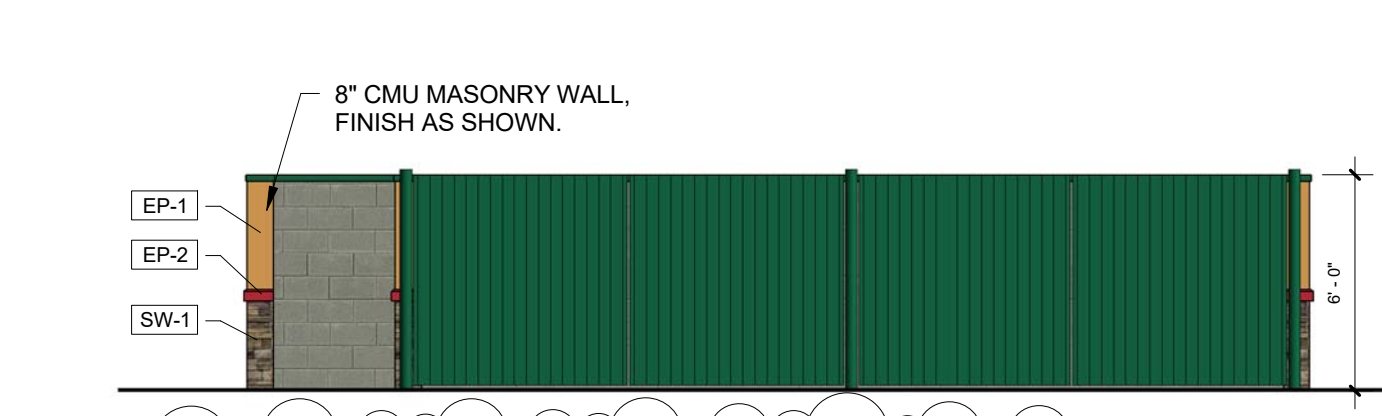
6 DUMPSTER ENCLOSURE - ELEVATION SOUTH A-2 3/16" = 1'-0"
