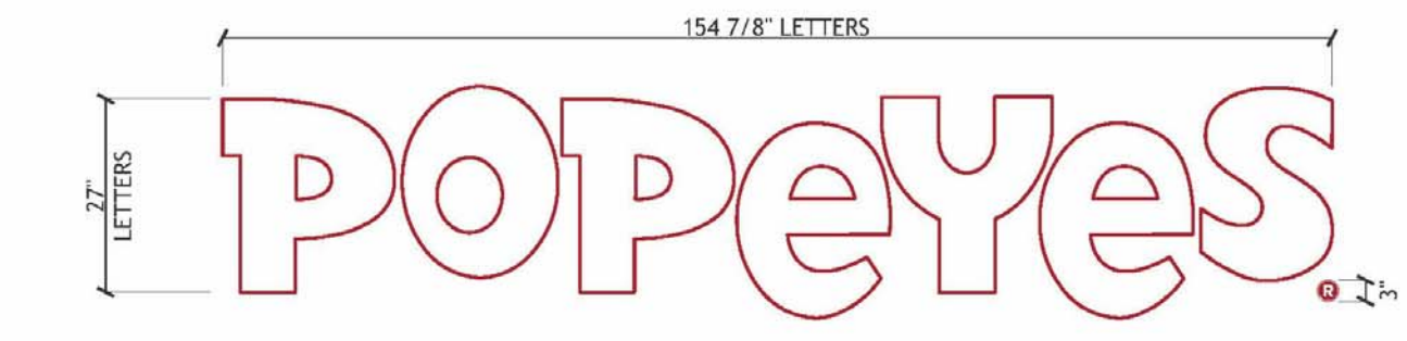
1 ILLUMINATED CHANNEL LETTERS FRONT VIEW AREA: 29.04 SQ FT SCALE: 1/2" = 1'-0"
