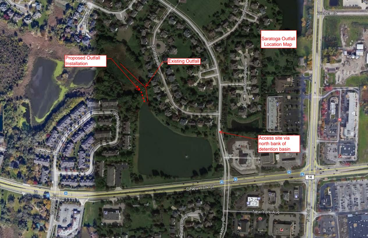
Earth Excavation, Excavate Approximately 100' of 3' flat bottom swale with 3:1 side slopes, Spoils to be bermed onsite, approximately 2' deep
