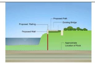
Aurora Riverwalk - Proposed Cross Section at Replacement of the Existing Pedestrian Walkway Rotary Bridge – <u>Option 2</u>
