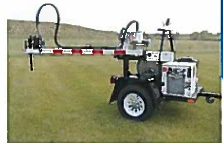
The extended reach ERV-750 valve exerciser allows valve operation from the roadside.
