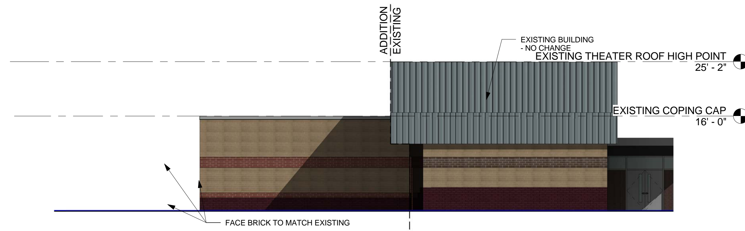
3 EAST ELEVATION - BLACK BOX ADDITION 1" = 10'-0"
