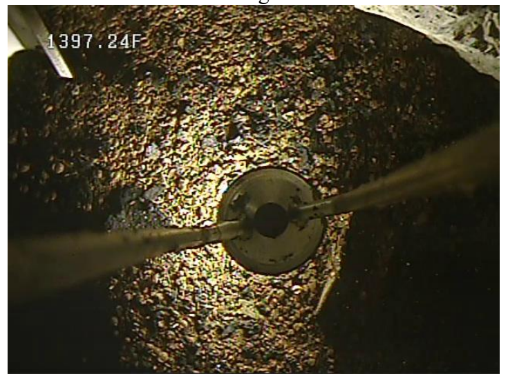
1397' Bottom settled scale/sand, soft
