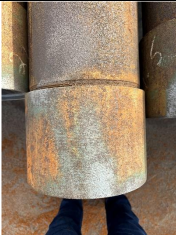
Improper thread engagement and stretched threads
