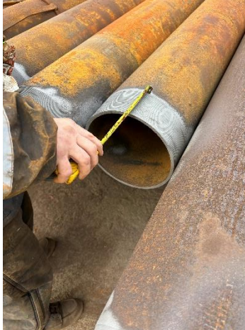
J. Kopp inspecting thread engagement depth
