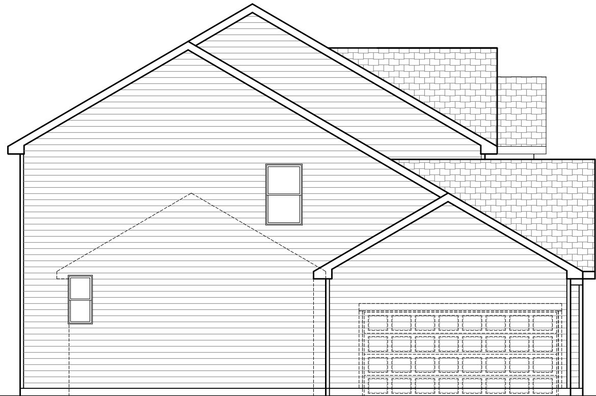
OPT. 2 CAR SIDELOAD W/1 CAR FRONT LOAD GARAGE LEFT SIDE ELEVATION
