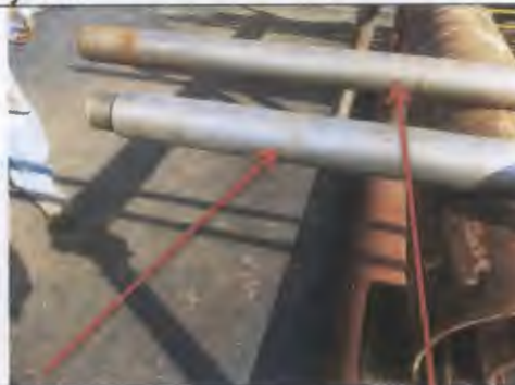
Heavy scouring at seal location on top shaft. Lower shaft has some wear at bearing journals.
