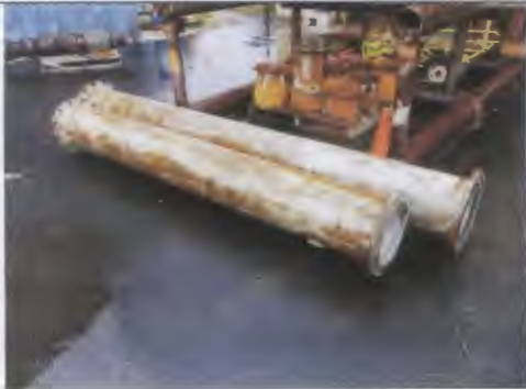
NP3 flanged column pipe racked in Layne yard. One 10' length, one 8' 3 1/4" length.
