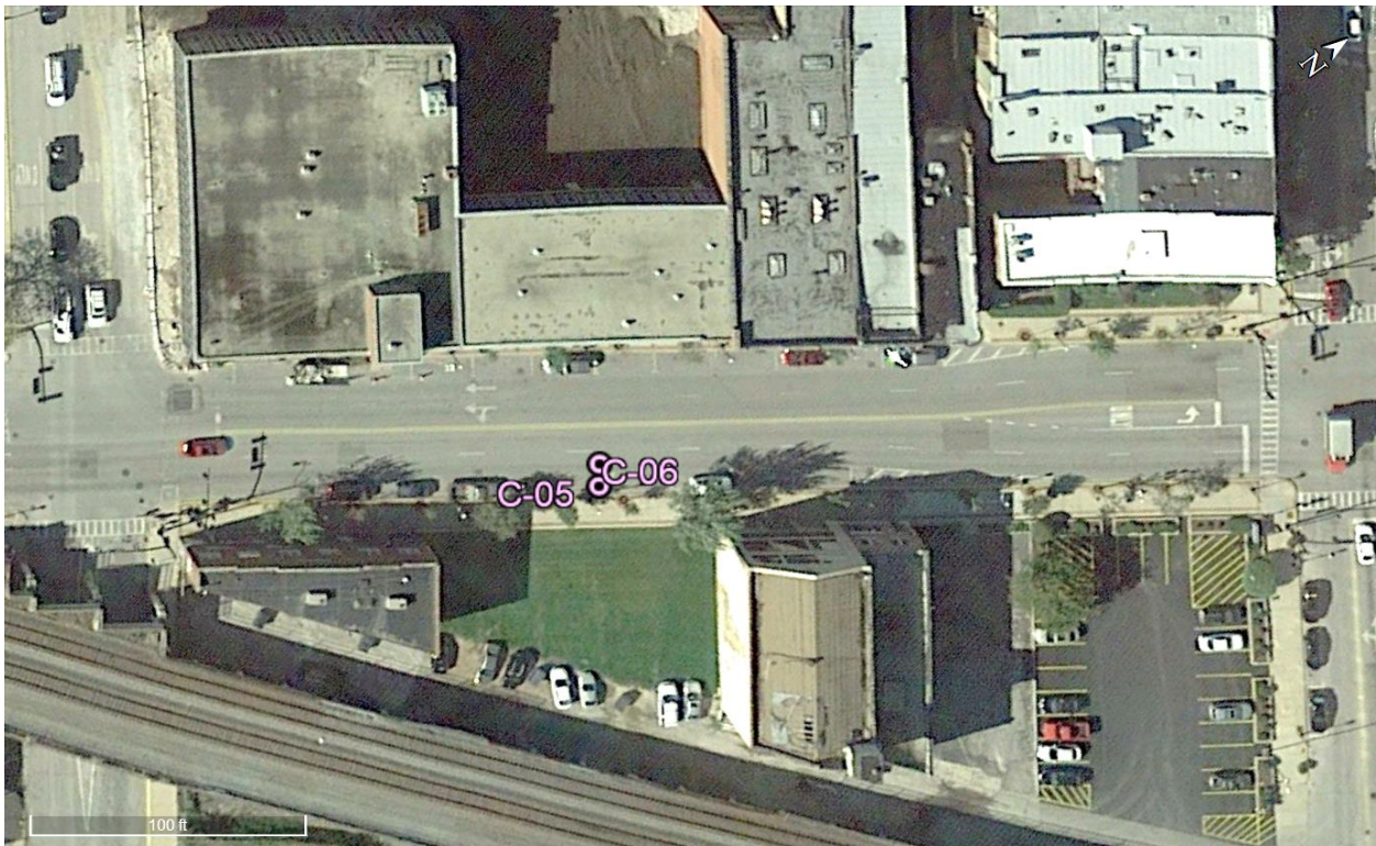
Exhibit 3) Showing one pavement core in the drive lane and one pavement core in the parking lane on the east side of Broadway Avenue between Downer Place and Benton Street
