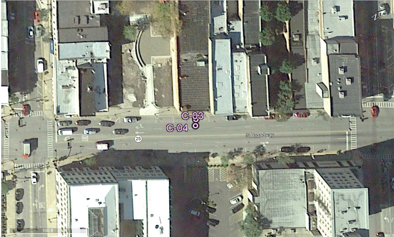
Exhibit 2) Showing one pavement core in the drive lane and one pavement core in the parking lane on the west side of Broadway Avenue between Galena Boulevard and Downer Place
