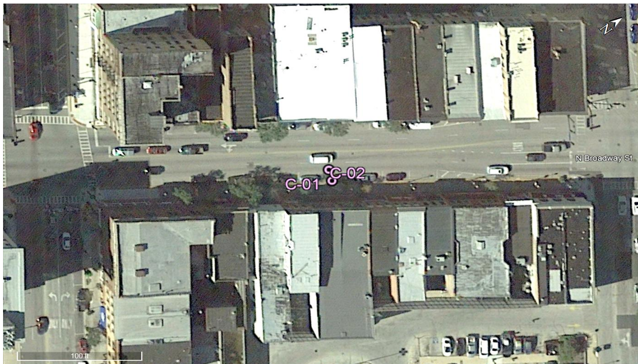
Exhibit 1) Showing one pavement core in the drive lane and one pavement core in the parking lane on the east side of Broadway Avenue between New York Street and Galena Boulevard
