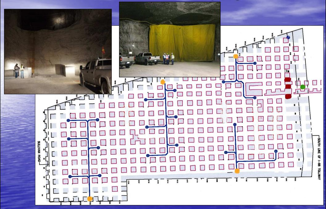
In-Mine: Injection Wells, Distribution Piping, Bulkheads, Extraction Well
