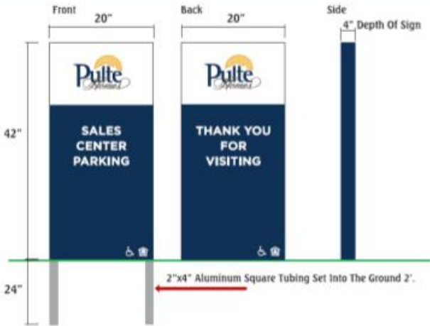
42"x20" Custom Made Aluminum Box Sign w/Aluminum Square Tubing Frame. Sign is 4" Deep w/Front, Back & Side Faces Made Out Of .063 Aluminum Painted PMS 540. White Vinyl Lettering & Digitally Printed Logo To The Front & Back.
