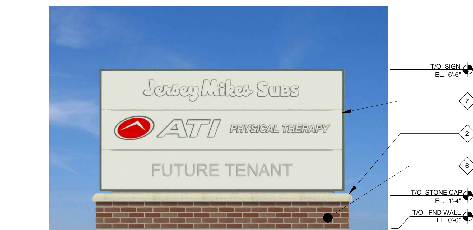
4 MONUMENT SIGN - FRONT/BACK ELEVATION 1/2" = 1'-0"
