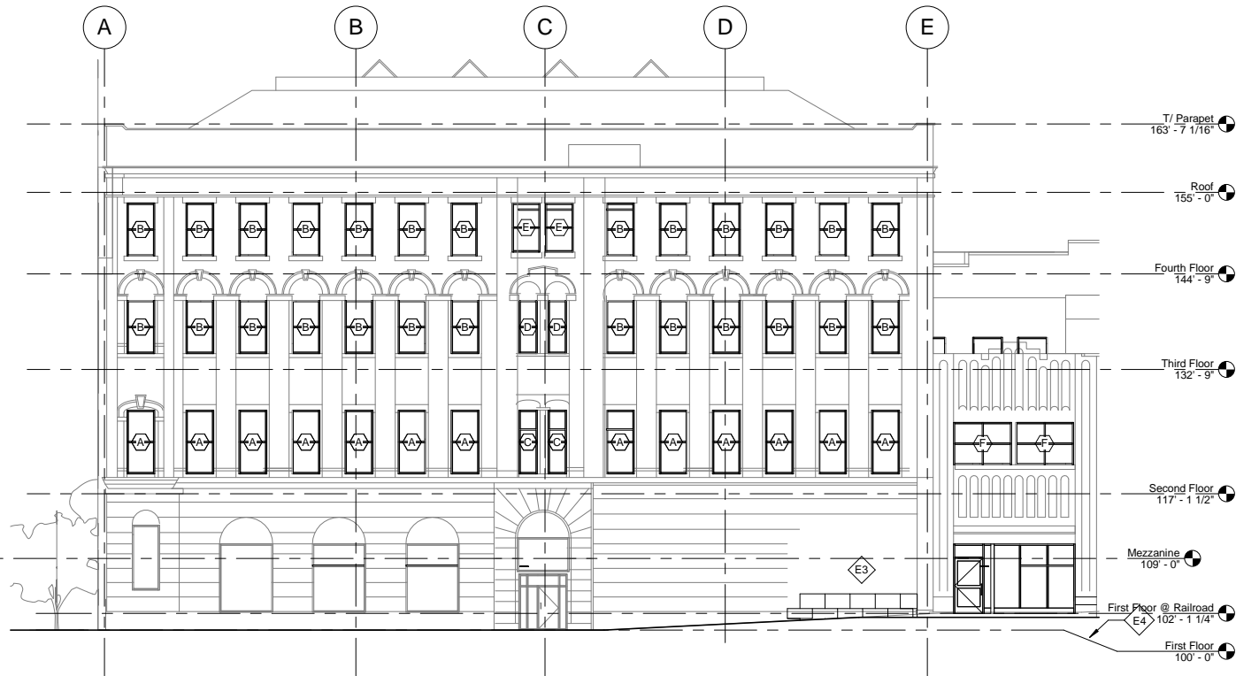
1 BUILDING ELEVATION - SOUTH 3/32" = 1'-0"
