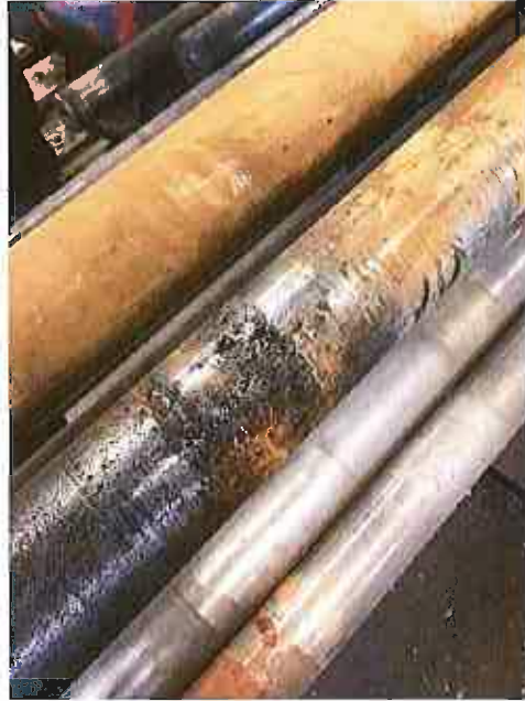
Heavy pitting on impeller shaft
